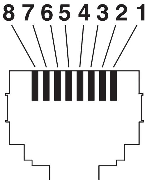
Connector pin assignment plug RJ45
