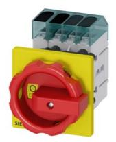
Load disconnector 3LD3, Iu 32 A Main switch 3-pole + N Rated operating capacity for AC-23 A at 400V 11.5kW Front plate mounting Basic switch with Central hole mounting 22.5mm Rotary actuator red / yellow 66 x 66 mm
