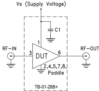
**Fig 1.** Block Diagram of Test Circuit used for characterization. (DUT soldered on Mini-Circuits Characterization test board TB-01-28B+) Gain, Return loss, Output power at 1dB compression (P1 dB), output IP3 (OIP3) and noise figure measured using Agilent’s N5242A PNA-X microwave network analyzer.
