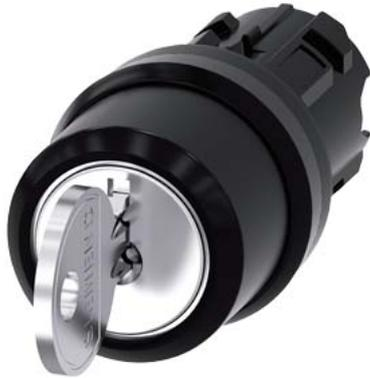
RONIS key-operated switch, 22 mm, round, plastic, lock number SB30, with 2 keys, 3 switch positions I>O<II, momentary contact on the left, latching on the right, actuating angle 2x45°, 10:30h/12h/13:30h, Key removal O+II, possible special locks: SB31, 421, 455 Z=50-unit packaging
