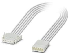
Assembled PCB connector / Connecting cable with 2 printed circuit board connectors, rated current: 6 A, cable length: Free input (0.1 ... 3.0 m), Head 1: 4-position , pitch: 2.5 mm , Crimp connection , Socket, Color: white, Cable type: Individual litz wire, PVC, 22 AWG, white, Head 2: 4-position, pitch: 2.5 mm , Crimp connection , Pin, Color: white, Cable type: Individual litz wire, PVC, 20 AWG, white, Individual litz wire, PVC, 22 AWG, white
