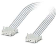
Assembled PCB connector / Connecting cable with 2 printed circuit board connectors, rated current: 6 A, cable length: Free input (0.1 ... 3.0 m), Head 1: 4-position , pitch: 2.5 mm , Crimp connection , Socket, Color: white, Cable type: Individual litz wire, PVC, 22 AWG, white, Head 2: 4-position, pitch: 2.5 mm , Crimp connection , Socket, Color: white, Cable type: Individual litz wire, PVC, 20 AWG, white, Individual litz wire, PVC, 22 AWG, white
