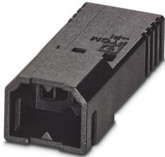
PCB connector, nominal cross section: 0.75 mm<sup>2</sup>, color: black, nominal current: 6 A, rated voltage (III/2): 160 V, contact connection type: Pin, number of potentials: 4, number of rows: 1, number of positions: 4, number of connections: 4, product range: PTCM 0,5/..-PI, pitch: 2.5 mm, connection method: Crimp connection, conductor/PCB connection direction: 0 °, plug-in system: COMBICON PTSM, locking: Snap-in locking, mounting: Engagement nose, type of packaging: packed in cardboard
