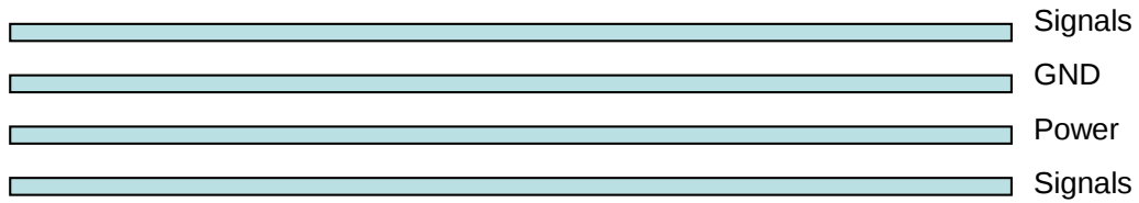
Figure 17: Typical 4-layer PCB construction
