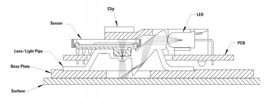
Figure 2. Sectional view of PCB assembly highlighting all optical mouse components (optical mouse sensor, clip, lens, LED, PCB, and base plate).
