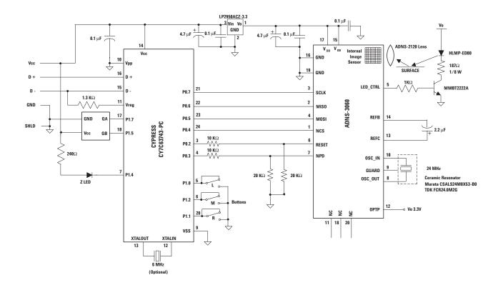
Figure 1. Circuit-level block diagram for ADNK-3061 designer's kit optical mouse using the Agilent ADNS-3060 optical mouse sensor and Cypress CY7C63743-PC enCoRe USB Controller.
