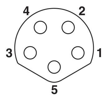
Pin assignment of M8 socket, 5-pos., B-coded
