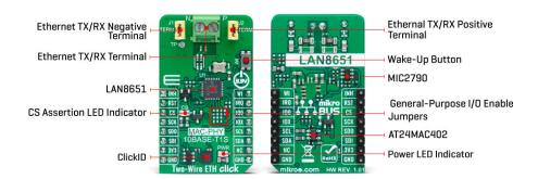
The integrated PHY of the LAN8651 allows for creating both multidrop and point-to-point network topologies, with up to 25m maximum in length for a point-to-point network. The multidrop mode supports up to at least 8 PHYs connected to a common mixing segment of up to at least 25m in length. The ability to connect multiple PHYs to a common mixing segment reduces weight and implementation costs by reducing cabling and switch ports.
