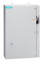
Reversing motor starter Size 2 1/2 Three phase full voltage Solid-state overload relay OLRelay amp range 25-100A 110V 50HZ / 120V 60HZ coil Combination type 100A circuit breaker Encl NEMA type 4X 304 S-steel Water/dust tight noncorrosive
