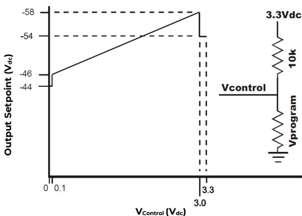
An open circuit on this pin reverts the voltage level back to the original setting.
