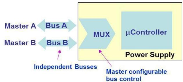
Diagram showing the dual I<sup>2</sup>C bus system.
