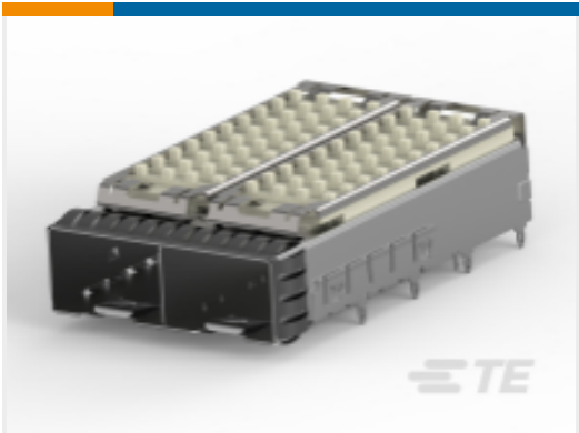
TE Part # 2198230-1 SFP+ Enhanced 1x2, PCI Heatsink
