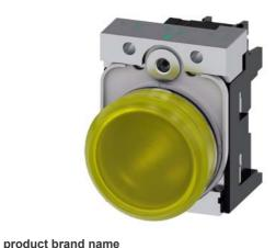
Indicator lights, 22 mm, round, Metal, shiny, yellow, lens, smooth, with holder, LED module with integrated LED 230 V AC, screw terminal, with laser labeling, inscription or symbol Customer-specific selection with SIRIUS ACT configurator (CIN)
