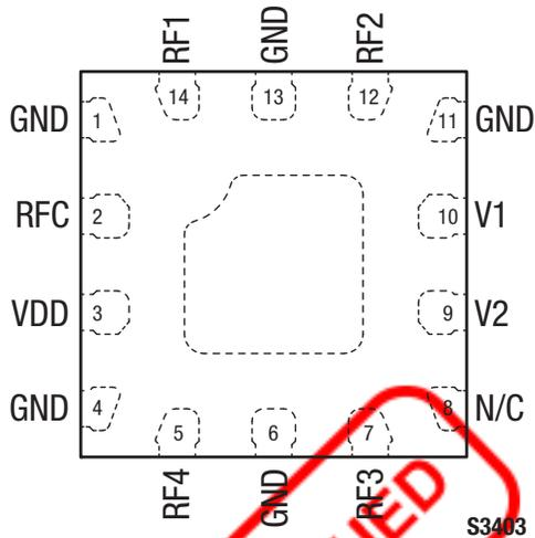
Figure 2. SKY13524-639LF Pinout – 14-Pin QFN (Top View)
