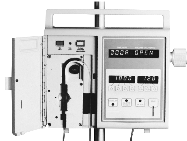
MML medical application. Intranavenous fluid flow controller automatically dispenses fluids for medications, therapy, and nutrition.
