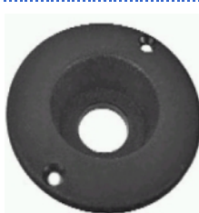
SRP-1 Recess Plate Moulded in black, (as standard), white or grey plastic and designed to allow a flush mounting on the front of a cabinet for our S2 and S4 jack sockets. This recess plate can also be used for lamps and switches etc. for enhancing the external appearance of cabinets and entertainment equipment. Made with a matt, non reflective surface finish. CL1396 SRP-1. Weight 2.8 Kg. per 1000.
