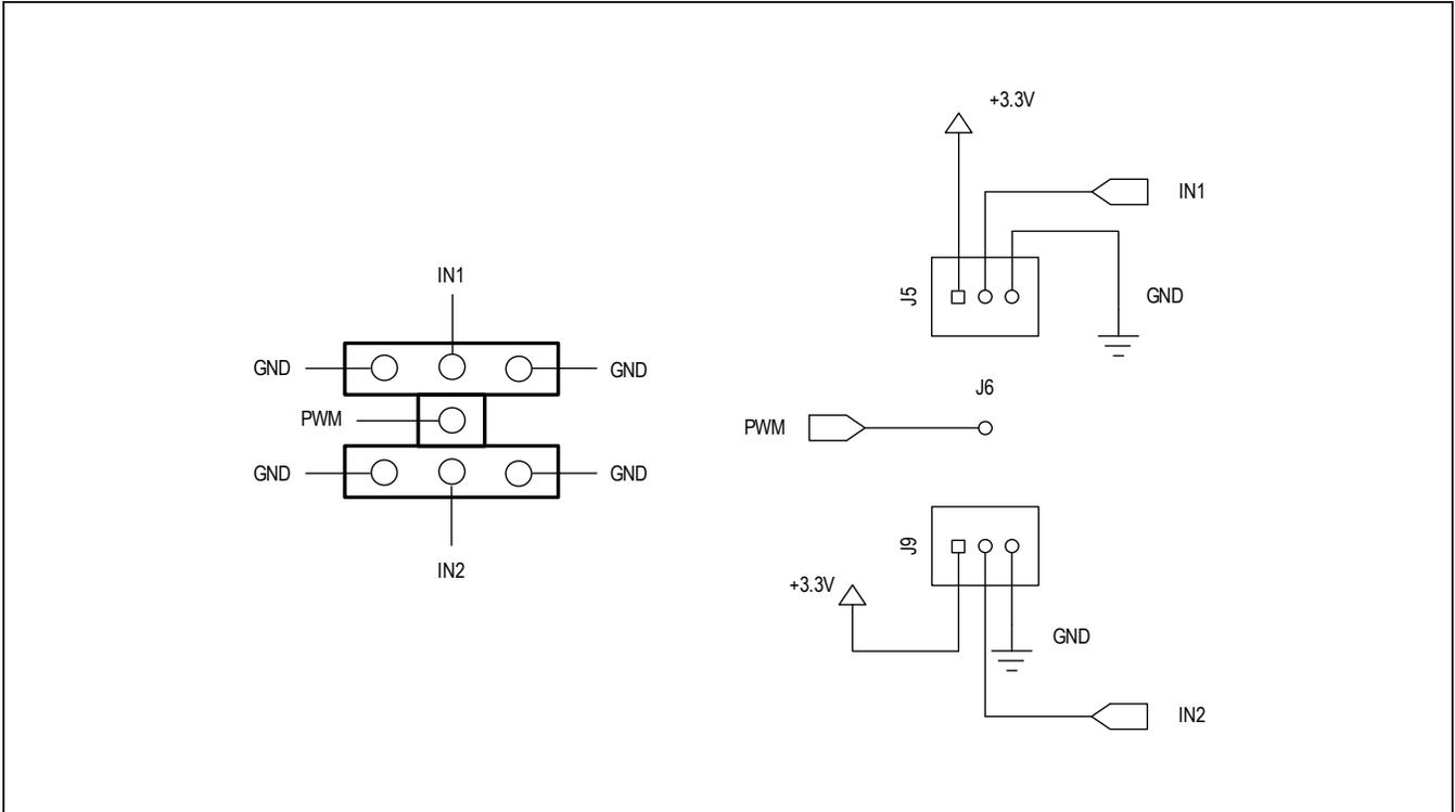
Figure 2. Configuration of the MAX22207 Input Headers J5, J6, and J9
