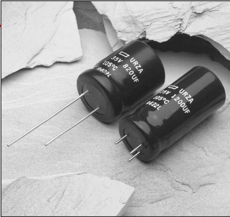
The URZA series capacitors are designed for high frequency applications, switching power supplies for example. These capacitors have a rated load life of 5,000 hours and an operating temperature of  $-55^{\circ}\text{C}$  to  $+105^{\circ}\text{C}$  for 6.3 to 100 volt products and  $-40^{\circ}\text{C}$  to  $+105^{\circ}\text{C}$  for 160 to 250 volts. The URZA series is available in 2 and 3 lead radial mount or optional 3rd lead axial mount.
