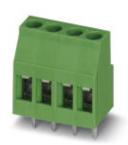
PCB terminal block, Nominal current: 24 A, Nom. voltage: 400 V, Pitch: 5 mm, Number of positions: 6, Connection method: Screw connection, Mounting: Soldering, Conductor/PCB connection direction: 0 °, Color: green, The article can be aligned to create different nos. of positions!
