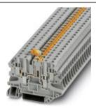
Knife disconnect terminal block, nom. voltage: 500 V, nominal current: 20 A, connection method: Screw connection, number of connections: 4, cross section:0.14 mm² - 6 mm², AWG: 26 - 10, width: 6.2 mm, color: gray, mounting type: NS 35/7,5, NS 35/15
