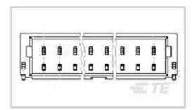
PCB Connector Assembly Type: PCB Mount Header
