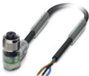
Sensor/actuator cable, 4-position, PVC, gray RAL 7001, free cable end, on Socket angled M12, A-coded, with 2 LEDs, cable length: 5 m
