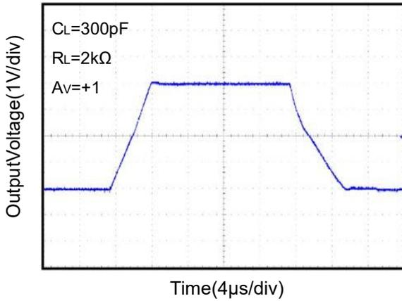
VLarge Signal Transient Response at +2.5V
