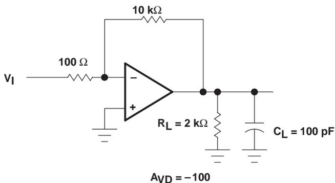
Figure 2. Inverting Amplifier
