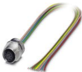
Sensor/actuator flush-type socket, 8-pos., M12, A-coded, front/screw mounting with M16 thread, with 1 m TPE litz wire, 8 x 0.25 mm 2 , VPE 250
