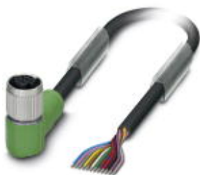
Sensor/actuator cable, 12-position, PUR halogen-free, black RAL 9005, free cable end, on Socket angled M12 SPEEDCON, A-coded, cable length: 3 m
