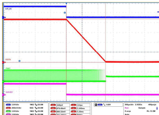
Figure 8-9. Soft-stop channel A (0 ms TOFF_DELAY)
