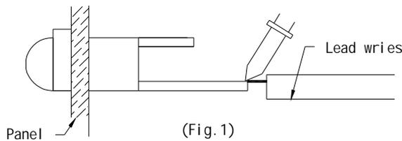
2) When soldering wire to the lead, work with a Fig (See Fig.2) to avoid stressing the package.
