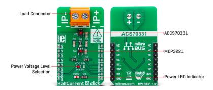
The ACS70331 offers a sensitivity of 200mV/A, capable of measuring currents from -5A to +5A. With an operating range of approximately 1MHz, the sensor provides fast output voltage variations in response to changes in the load current, without noticeable latency. The output voltage is then processed by the MCP3221 ADC, allowing digital data to be accessed via the I2C interface.
