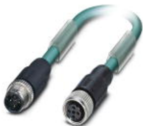
Bus system cable, Ethernet CAT5, 4-position, PUR halogen-free, water blue RAL 5021, shielded, Plug straight M12, coding: D, on Socket straight M12, coding: D, cable length: 8 m, Crossover
