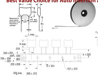
Type CDA15 is designed especially for auto-insertion and is the best value choice for tape and reel and ammo-pack feed systems. CDA15 is used in commercial and industrial applications requiring high stability, high Q and close capacitance tolerances. Type CDA15 T max is ideal for tuned circuits, delay lines and filter circuits.
