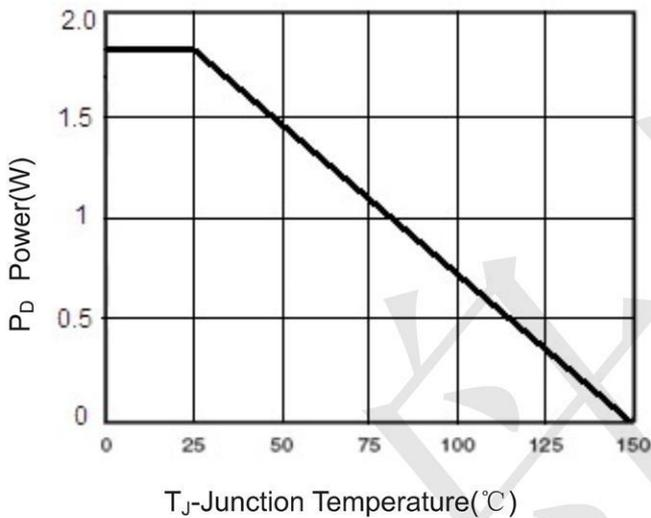
Figure 3 Power Dissipation
