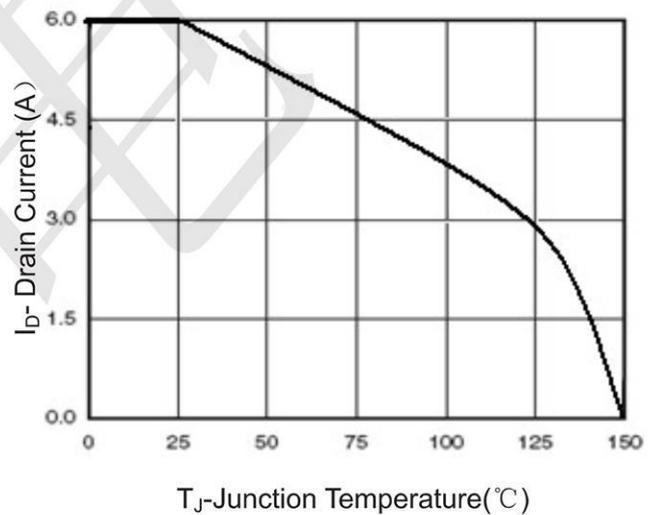
Figure 4 Drain Current
