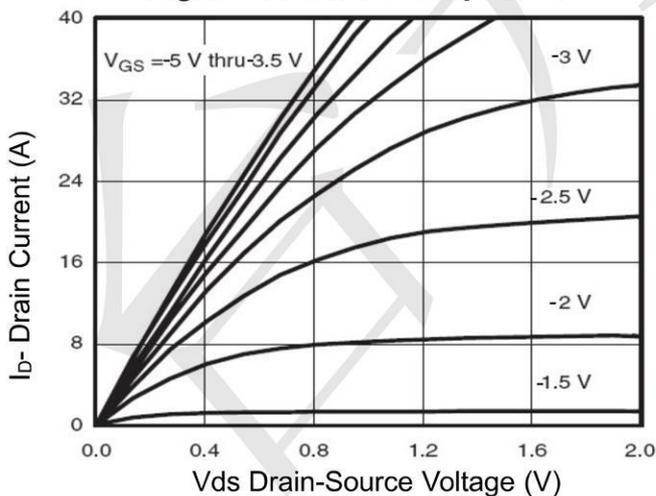
Figure 5 Output Characteristics
