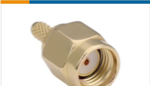
TE Part #CONREVSMA007-G RP-SMA Plug 50 Ohm Cable Crimp
