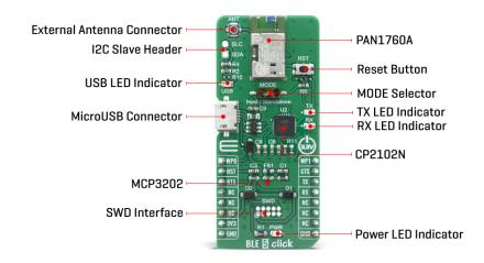
The BLE 5 Click in AT-Command or Host mode Click board™ Besides the commonly used UART RX, TX, RTS, and CTS, BLE 5 Click has also WPO and WP1 pins, which are routed to the PWM and AN pins of the mikroBUS™ socket, respectively. The PAN1760A modul contains internal antenna with receiver sensitivity -93 dBm, and the BLE 5 click board also features an SMA connector so it can be equipped with the appropriate 2.4 GHz antenna.
