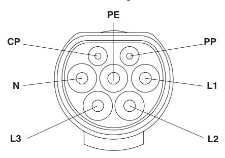
Pin assignment of the Vehicle Connector
