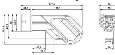
Make sure that the vehicle charging connector is placed in an appropriate charging connector holder, which ensures a minimum protection rating of IP24 in accordance with IEC 61851-1, for the entire time between charging. To create this charging connector holder, use the dimensions of the vehicle charging connector. Detailed dimensions can also be found in the Download area.
