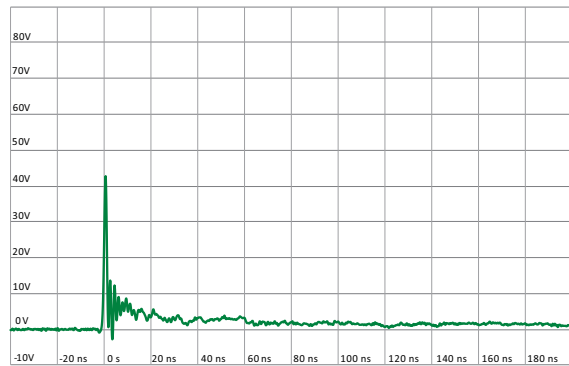
IEC 61000-4-2 +8 kV Contact ESD Clamping Voltage
