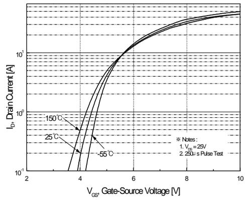
**Figure 2. Transfer Characteristics**
