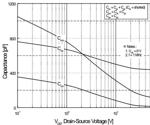
**Figure 5. Capacitance Characteristics**
