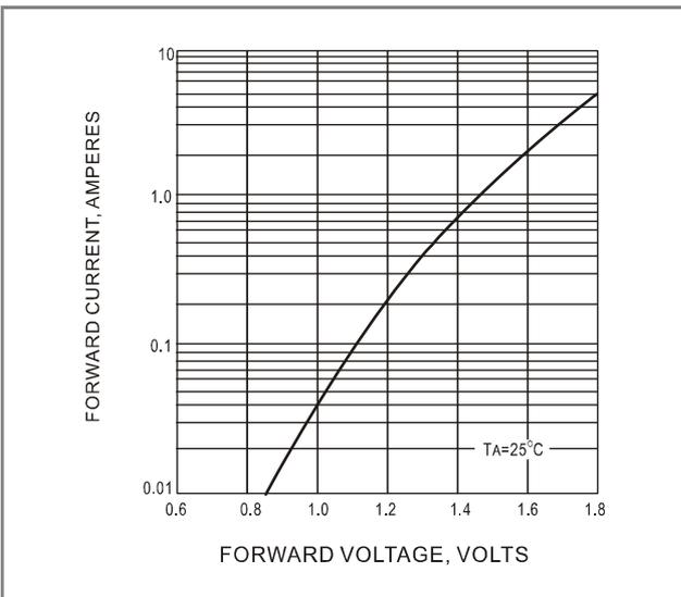
Fig. 3 FORWARD CHARACTERISTICS
