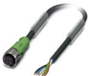
Sensor/actuator cable, 5-position, PUR halogen-free, black-gray RAL 7021, free cable end, on Socket straight M12 SPEEDCON, A-coded, cable length: 2 m
