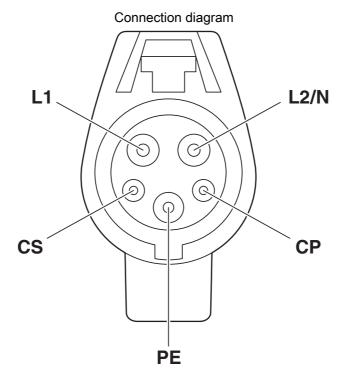
Pin assignment of the Vehicle Connector
