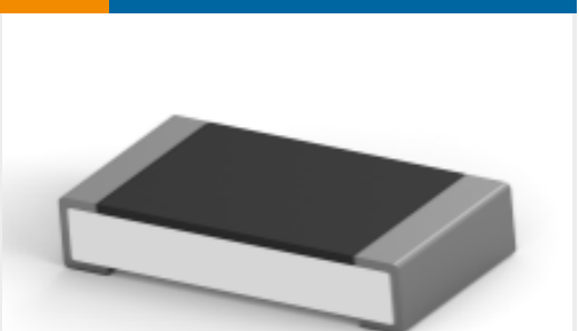
TE Part #1-2176388-8 RQ 1206 15R 0.1% 10PPM 5K RL
