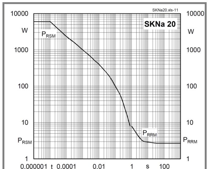
Fig. 11 Reverse power dissipation vs. time
