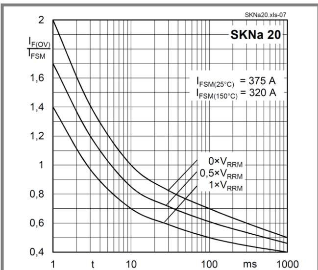
Fig. 7 Rated surge overload current vs. time
