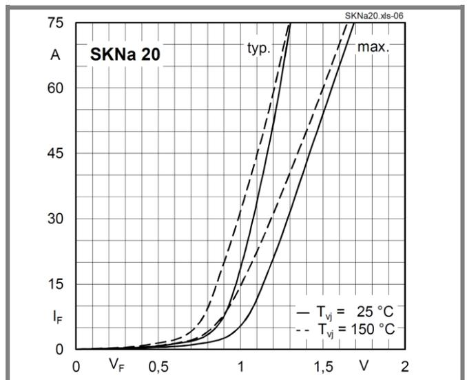
Fig. 6 Forward characteristics
