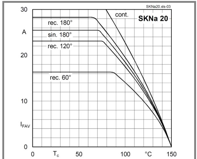
Fig. 3 Forward current vs. case temperature
