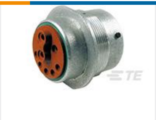
TE Part #HD34-24-91PN REC, 9P, AL, N, 8/12/16, P
