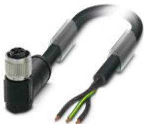
Power cable, 3-position, PVC, black, free cable end, on Socket angled M12, S-coded, cable length: 1 m, for AC current up to 16 A/230 V
