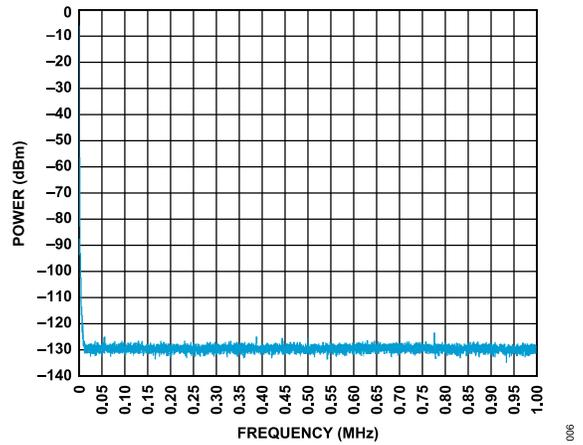
Figure 6. Analog Input Acquisition Spectrum to 1 MHz
