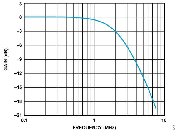
Figure 8. ADC and DAC Filter Composite Response
