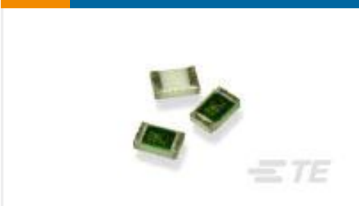
TE Part #1-1879217-2 CPF 0603 390K 0.1% 25PPM 1K RL
