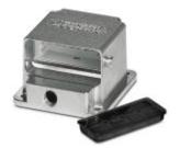
Connector on motor side, EMC metal housing attachment incl. crimp contact insert, with flat seal and coated protective cover, without crimp contacts, housing with coatable thick-layer passivation
