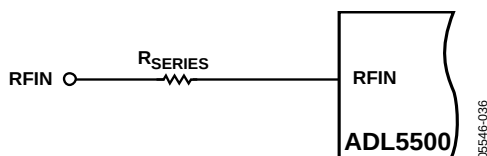
Figure 36. Attenuating the Input Signal
