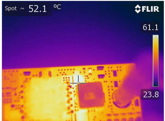
Figure 30. Thermal Image of SR1 at 48 V<sub>DC</sub> Input, 6 A Load, No Airflow, 1 Hour Soaking Time
