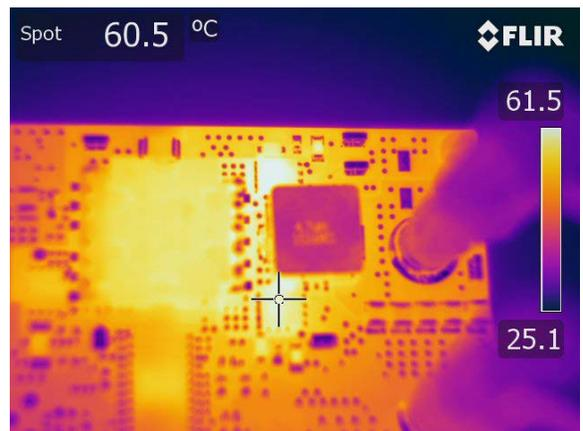
Figure 31. Thermal Image of SR2 at 48 V<sub>DC</sub> Input, 6 A Load, No Airflow, 1 Hour Soaking Time
