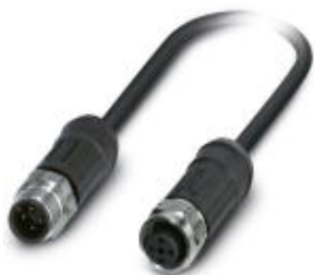
Sensor/actuator cable, 4-position, PE-X, black-gray RAL 7021, Plug straight M12, A-coded, on Socket straight M12, A-coded, cable length: 1 m, for outdoor applications, with high-grade steel knurl
